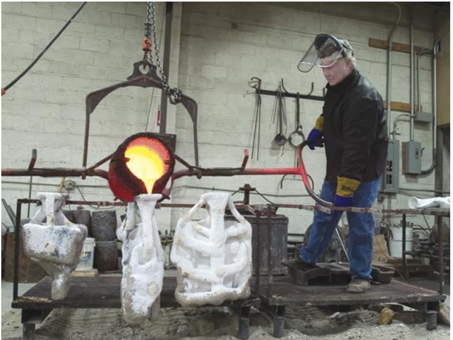
BELOW: ART FOUNDRY OWNER Alan Osborne DEMONSTRATES BRONZE CASTING OF NATHAN OLIVIERA SCULPTURE. PHOTO: DAVID M. ROTH
